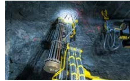
The bolting unit on the Boltec M has been optimized to reduce the overall feed length by 100 mm when compared to earlier bolting unit designs.
